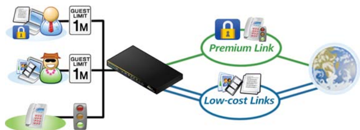
Traffic can be routed by application type using Advanced QoS and Outbound Policy
